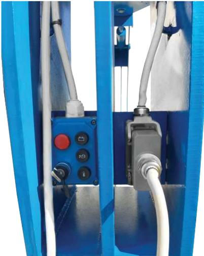
All hydraulic functions are controlled by a wired controller and a wireless system to ensure greater operator safety.
