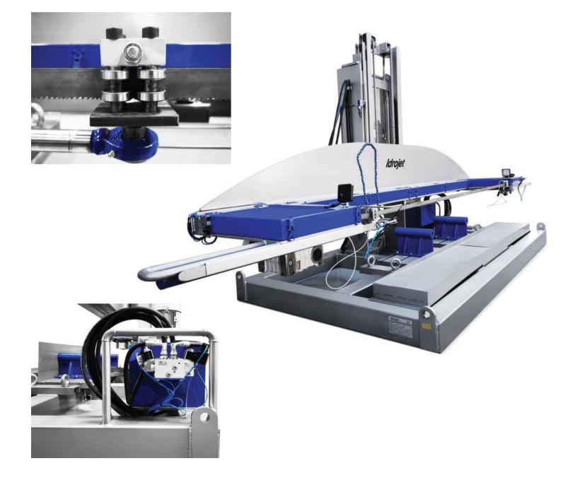
The cutting system has an assisted and automatic descent, to make the cuts safely.
