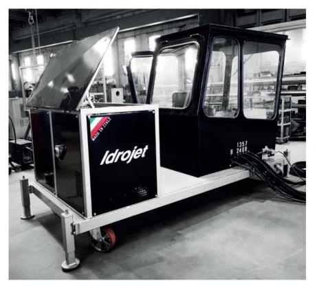
tubes with a maximum of 2 rotating lances on a cleaning site or "insitu", thanks to a scissor.lift that it is able to lift this machine till 5 mt. high, and spray high pressure water jets moving both horizontal and vertical and rotating them up to 1400 bar (20000 psi) maxi working pressure.
