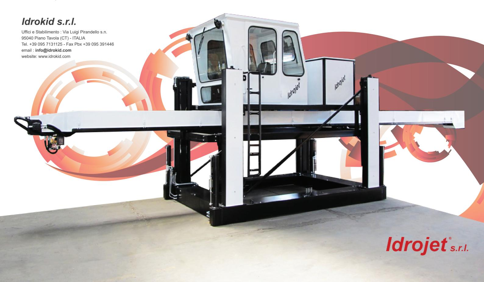
The internal cleaning robot mod. Autojet I 930-5 series 2015 is designed to clean all types and kinds of heat exchangers internal tubes. This robot works with a maximum of 5 rigid lances, which spray high pressure water, moving both in horizontally and vertically, up to 1400 bars (20,000 psi) max working pressure.(optional till 2800 Bars/36000 PSI)
