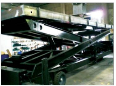
remote control box, and of course, the all machine is driven by an hydraulic power pack with an air explosion-proof engine for a better labour safety we built two models:
