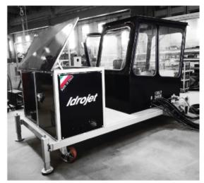
tubes with a maximum of 5 rotating lances on a cleaning site or "insitu", thanks to a scissor.lift that it is able to lift this machine till 5 mt. high, and spray high pressure water jets moving both horizontal and vertical and rotating them up to 1400 bar (20000 psi) maxi working pressure.
